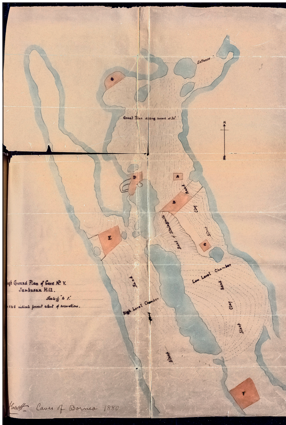
Figure 4: First known survey of a cave in Sarawak: 'Rough Plan of Cave No. V, Jambusan Hill' by A H Everett in 1878. Originally drawn at a scale of 1/16" to 1", the 'Entrance' is at top right leading to 'Great Talus dipping inward at 30° to a 'Bank of stalagmite' and two areas of 'Steep Clay Bank' in the 'Low Level Chamber' to the right, where excavations 'D', 'A', 'B', 'C' and 'F' are marked. Excavation 'E' is in the 'High Level Chamber' to the left, which also has a 'Steep Clay Bank'.
