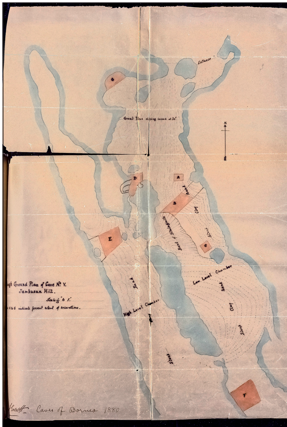
Figure 4: First known survey of a cave in Sarawak: 'Rough Plan of Cave No. V, Jambusan Hill' by A H Everett in 1878. Originally drawn at a scale of 1/16" to 1", the 'Entrance' is at top right leading to 'Great Talus dipping toward at 30° to a 'Bank of stalagmite' and two areas of 'Steep Clay Bank' in the 'Low Level Chamber' to the right, where excavations 'D', 'A', 'B', 'C' and 'F' are marked. Excavation 'E' is in the 'High Level Chamber' to the left, which also has a 'Steep Clay Bank'.
