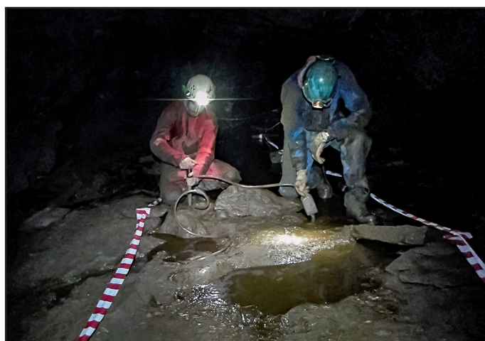
Figure 5: Drip-fed pool sampling. (Above): pool at Site 3, Ogof Draenen; (Below): sampling large pool at Site 4, Baker’s Pit. Pools being pumped with a bilge pump and the water passed through a filtering bottle to concentrate the sample.
