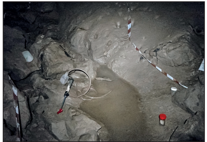
Figure 5: Drip-fed pool sampling. (Above): pool at Site 3, Ogof Draenen; (Below): sampling large pool at Site 4, Baker’s Pit. Pools being pumped with a bilge pump and the water passed through a filtering bottle to concentrate the sample.
