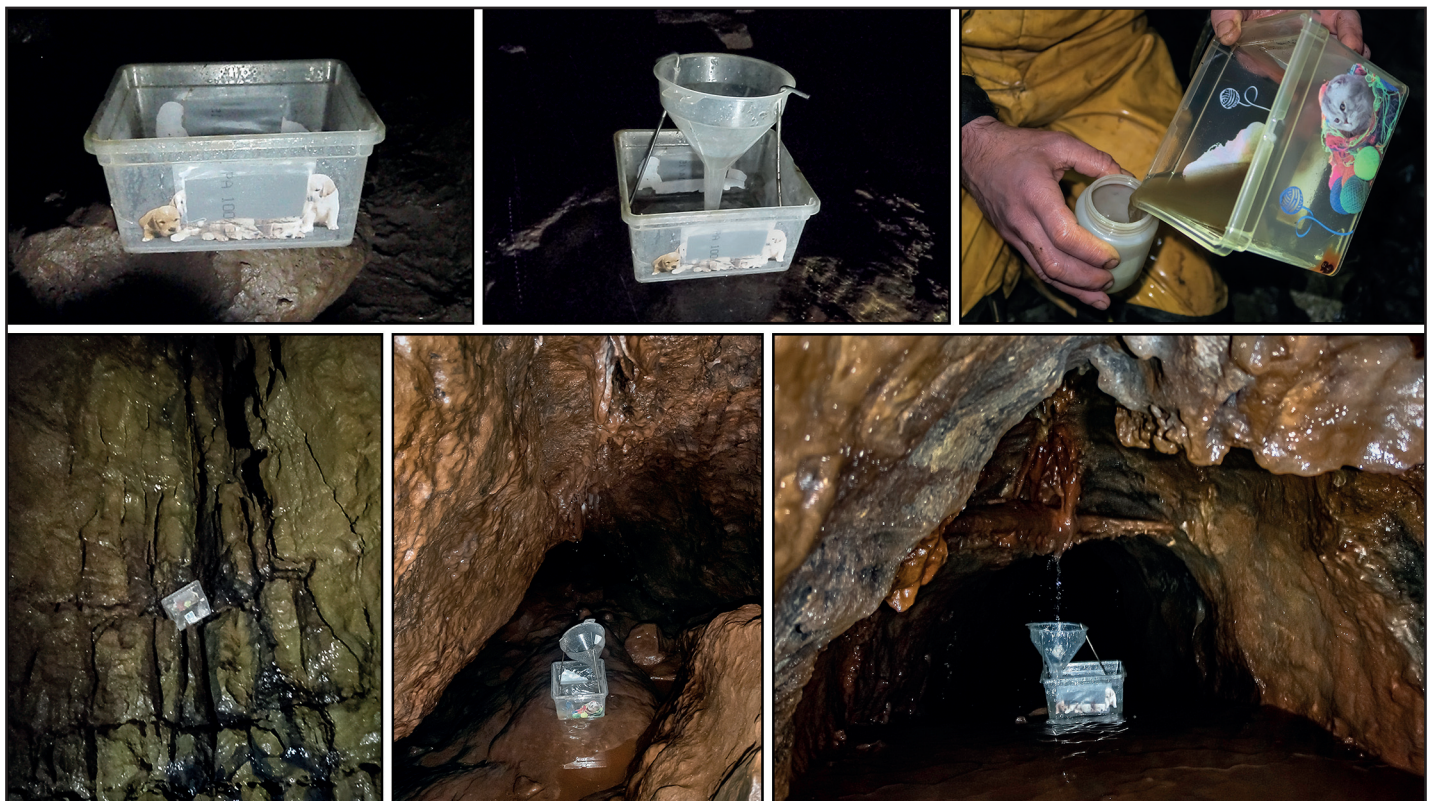
Figure 3: Trays used to sample dripping water. Top row (left to right): tray design, tray fitted with funnel, pouring sample into vial of preservative. Bottom row (left to right): Site 4, Ogof Draenen, tray without funnel wedged in fissure; Site 3, Baker's Pit, Site 1, Baker's Pit.
