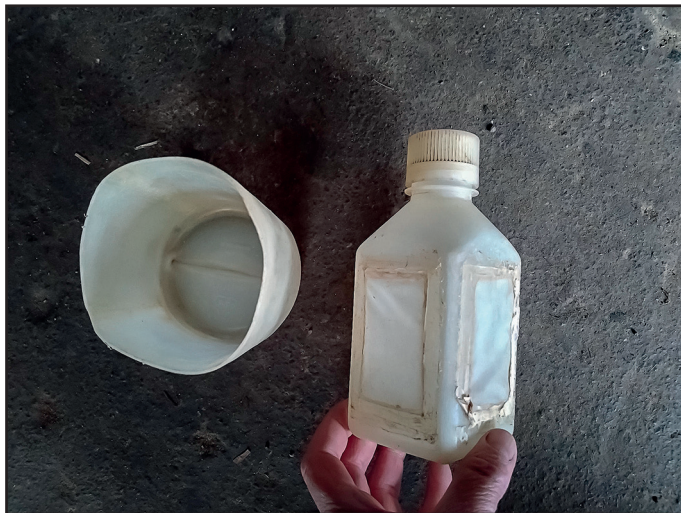
Figure 4: Filtering bottle (Brancelj, 2004) and bailing jug. The bottle has mesh-lined holes on two sides and can be carried inside the jug to protect the mesh screens during transportation between sampling sites.
