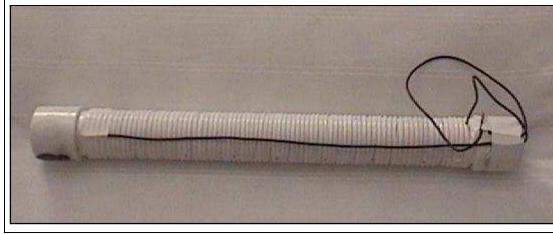
I chose to use the matching method of a series variable capacitor (a mica compression unit rather than a matching transformer or inductive link of one or more turns over the main coil. I think that this is a more efficient way of transferring the power to
