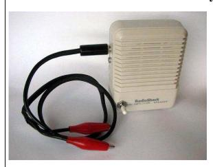
A small amplified speaker attached to the field telephone system can be a useful tool for Incident Command and other locations during a rescue. It allows personnel to receive information without constantly holding a phone to the ear. With this version, headphones can be connected and at the flip of a switch the speaker can be muted for privacy.
