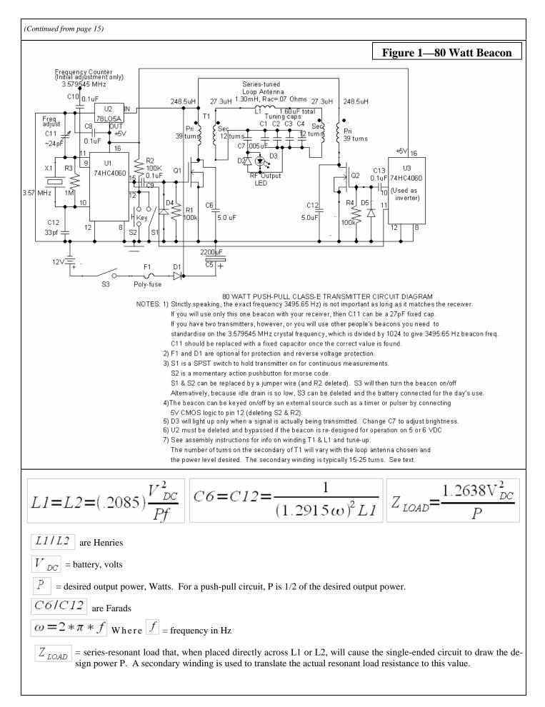
directly from the L1/L2 values and form a tuned "tank" circuit whose resonant frequency is offset from the beacon frequency by a specific amount. 5% capacitors are adequate for this low-Q circuit. The original single-ended equations are:
