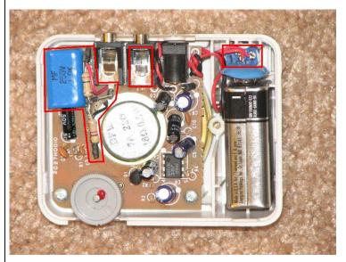
voltage ringer current. This is wired in series with the tip of the input jack as shown in the circuit diagram below. The external speaker (or headphones) jack is shown in the center highlighted area. It incorporates normally-closed switch contacts to disconnect the main speaker when a plug is inserted. I soldered a bridge across these contacts on the circuit board side (not visible in the photo) to enable the speaker to continue operating independently even when headphones are connected.
